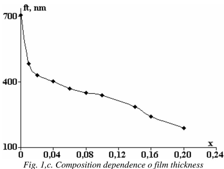
Fig. 1,c. Composition dependence of film thickness
