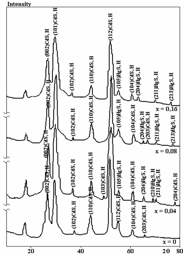
Fig. 2. X-ray diffractograms for  $x = 0, 0.04, 0.08$  and  $0.16$
