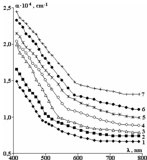
Fig. 3,a. Variation of absorption coefficient vs wavelength for seven representative film compositions. 1 -  $x = 0$ ; 2 -  $x = 0,01$ ; 3 -  $x = 0,04$ ; 4 -  $x = 0,06$ ; 5 -  $x = 0,1$ ; 6 -  $x = 0,16$ ; 7 -  $x = 0,2$
