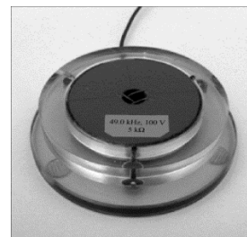
Fig. 5. Picture of piezoelectric motor ring used in experiments.
